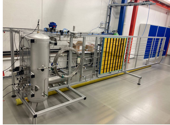
Figure 1: The setup of the gas system is shown. A dummy chamber, constructed with the same dimensions as the final modules of type-5, is mounted. For better visibility of the system, this picture shows the mechanical setup before the wiring was installed.
