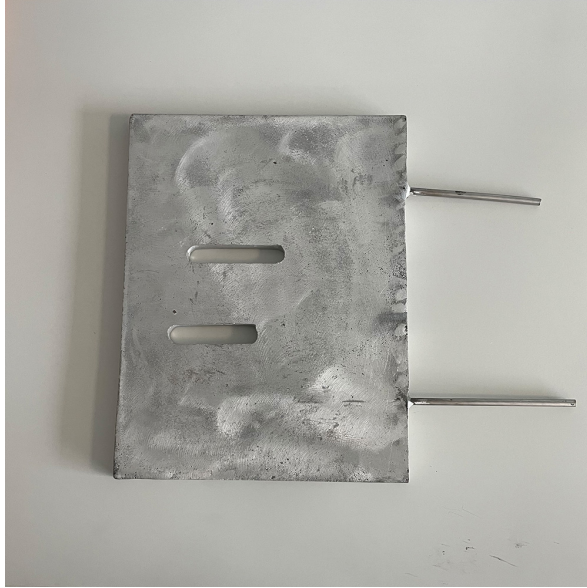
Figure 2: The new prototype - single aluminium plate with molded stainless steel pipe.
