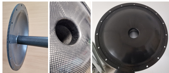
Figure 2: Joint of the window to the conical section ( outside view - left and inside view - middle). Window seen from the side attaching to the back wall of the target chamber (right).
