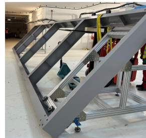
Figure 1: Manipulation tool for transport of frames through the tunnels of FAIR to the CBM cave (J. Thaufelder).
