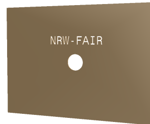
Figure 1: TGeoArbN-based geometry consisting of a simple iron plate with complex cut-outs (letters), directly extracted from the CAD model.
