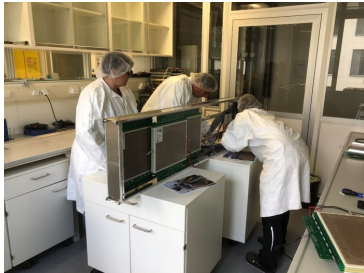
Figure 2: Module production in Heidelberg. A team of three technicians are building an M4 module.
