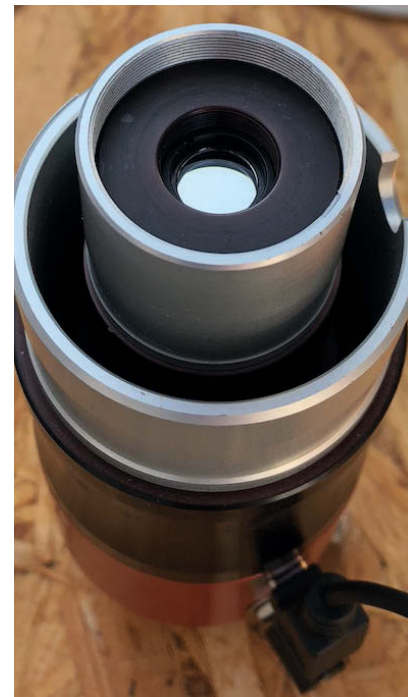
Fig. 6: The sunlight enters the filter system of the H \alpha QUARK eyepiece filter via this 12 mm bandpass filter (block filter), thus providing for dramatically reduced heat generation.
