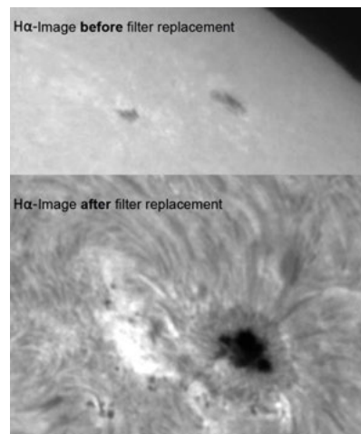
Fig. 5: An H \alpha image before and after replacement of the block filter. In the bottom picture, the numerous appearing structures characterizing the solar activity are clearly visible.
