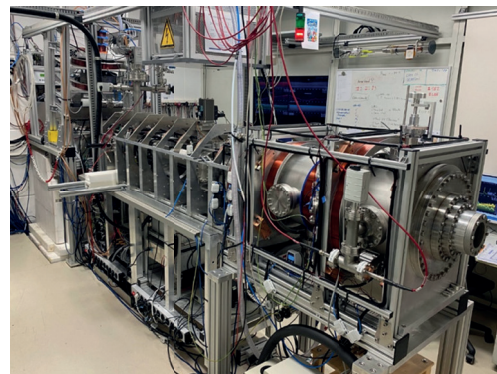
Fig. 1: The high-intensity positron beam at the ELBE centre for high-power beam source for defect characterisation and porosimetry
