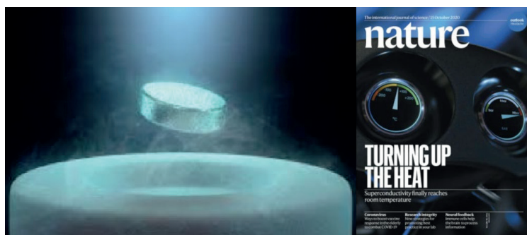
Fig. 1: A magnet flows over a cold superconductor and shows the Meissner effect.
