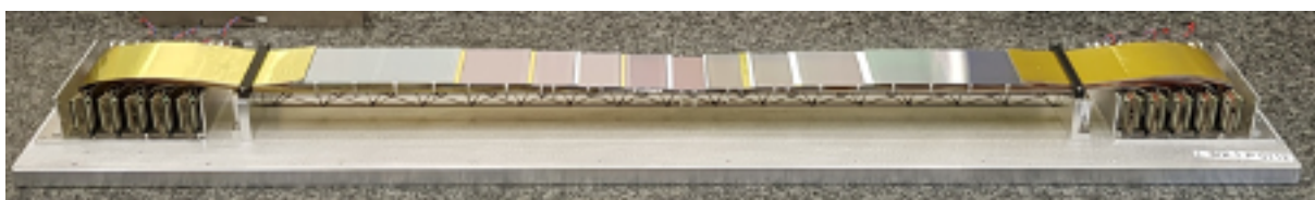
Figure 24: Detector ladder with 10 modules on a low-mass carbon fiber carrier
