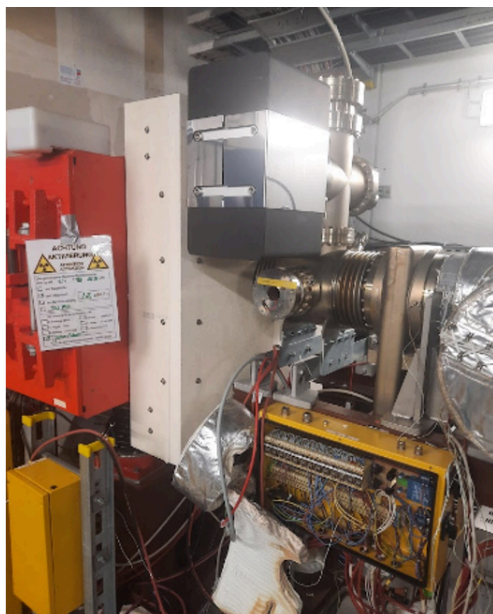
Figure 66: First cryogenic insert installed in SIS18 (stabilization of dynamic pressure)
