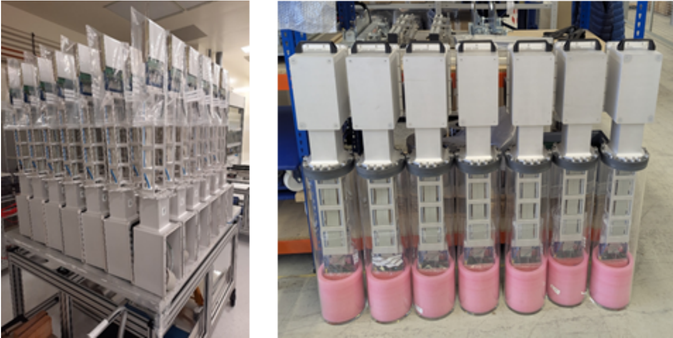
Figure 76: MWPC/IC detectors during pre-assembly (left) and fully assembled batch of 7 units (right).
