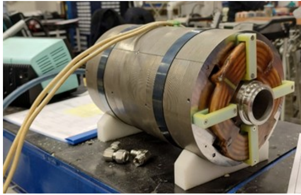
Figure 99: Quadrupole magnet prototype of the longest drift tube of cavity AIV, which was measured successfully in DC mode (E. Kuipers, Scanditronix)
