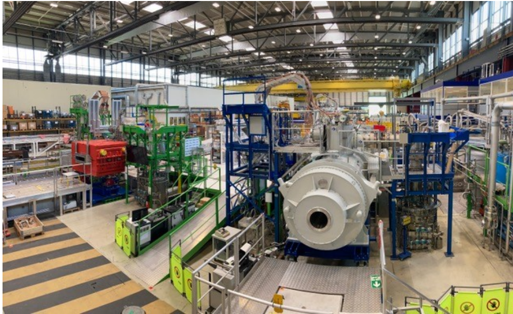
Figure 71: Superconducting dipole (left) and superconducting long multiplet (right) on testing benches at the testing facility at CERN.
