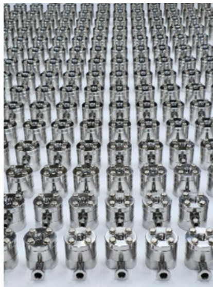
Figure 101: 400 drift tube heads for applying pre-vacuum and connecting the drift tubes to the cooling circuit (Hardcoats India, India)
