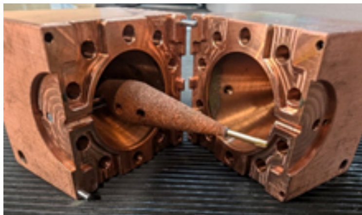
Figure 75: 3d-printed Fast Faraday-Cup
