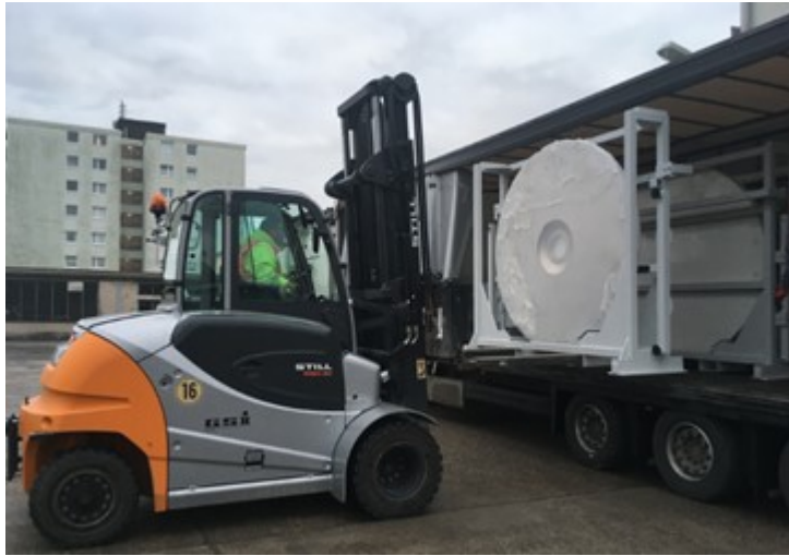
Figure 102: Unloading of the end plates and cavity sections of cavity AI (S. Mickat, GSI)
