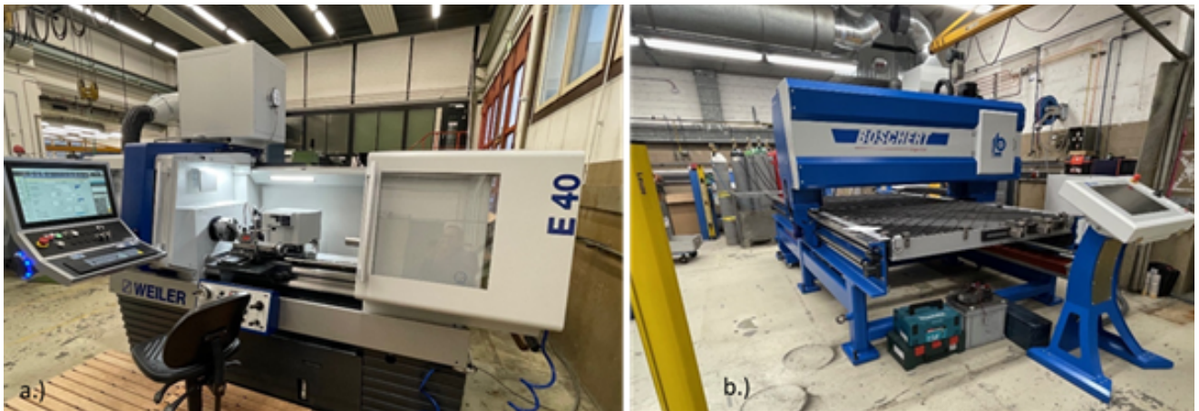
Figure 92: New machines in the Department of Mechanical Workshop and Metalworking. a.) shows the new lathe with combined drilling unit, b.) shows the plasma-cutting machine.
