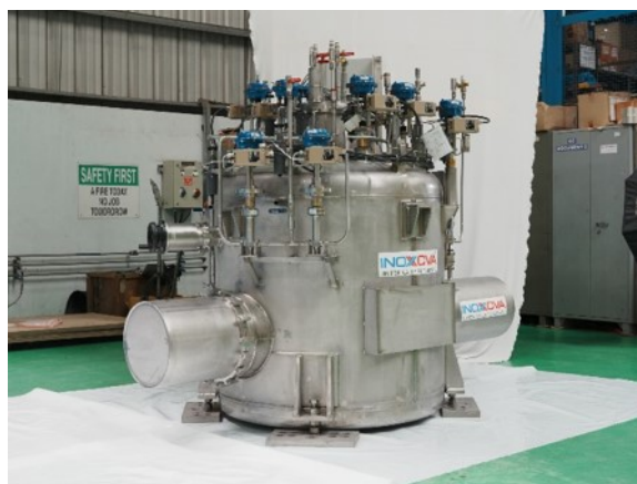
Figure 72: Local Cryogenics Feed-Box for the cryogenic branch at the entrance of Super-FRS.
