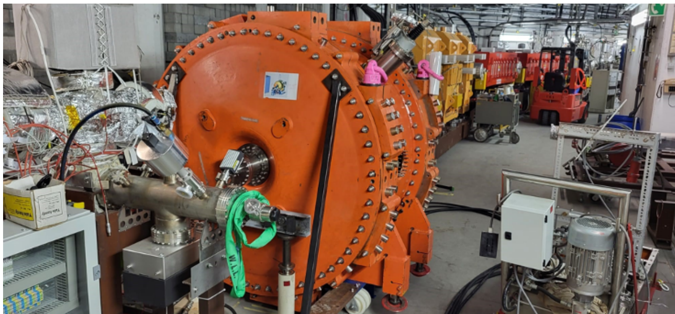
Figure 64: The new micro spill smoothing cavity at installation in SIS18
