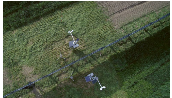
Experimental field site of Pillnitz (Dresden): MME instruments recording the microclimate at an agrivoltaic installation. Photo: Karl Wild
